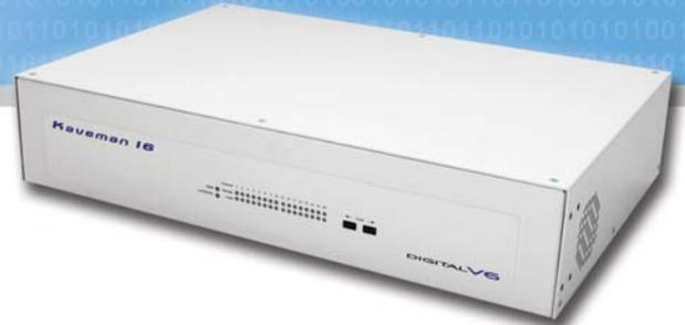
Since Kaveman is not a software-based solution, it does not consume valuable server resources and minimizes potential points of failure. This non-intrusive approach allows Kaveman to provide full keyboard, video, and mouse access for control right down to the BIOS level.
